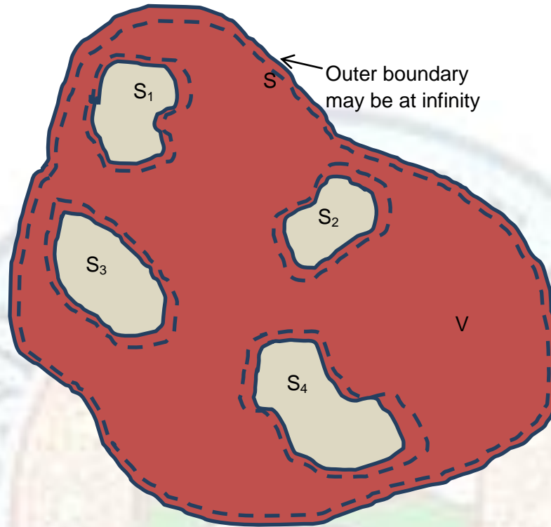
Fig. 2 Schematic of the conductors within a volume V.
