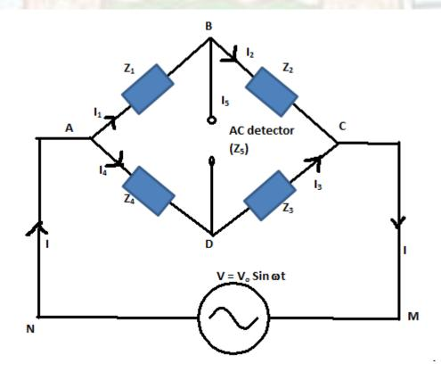
(iii) The impedance, present in the four arms of the bridge, need not be resistive impedances alone. They can, and, in general, include inductive and capacitive impedances also.
