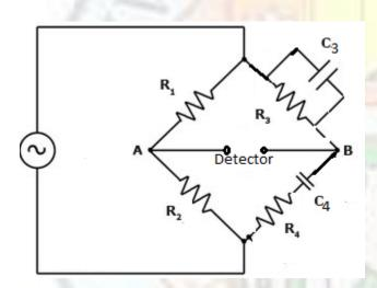
As seen in the diagram, this bridge has two resistors in the two arms of its Wheatstone bridge. There is (i) a combination of a resistor and a capacitor, in series, in one of the two arms and (ii) a combination, of a resistor and a capacitor, in parallel, in the fourth arm of this bridge.
