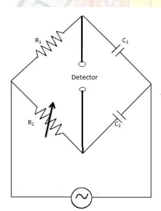
We start our discussion by analyzing two simple AC (Wheatstone) bridges, used for measurement of an unknown capacitance.
