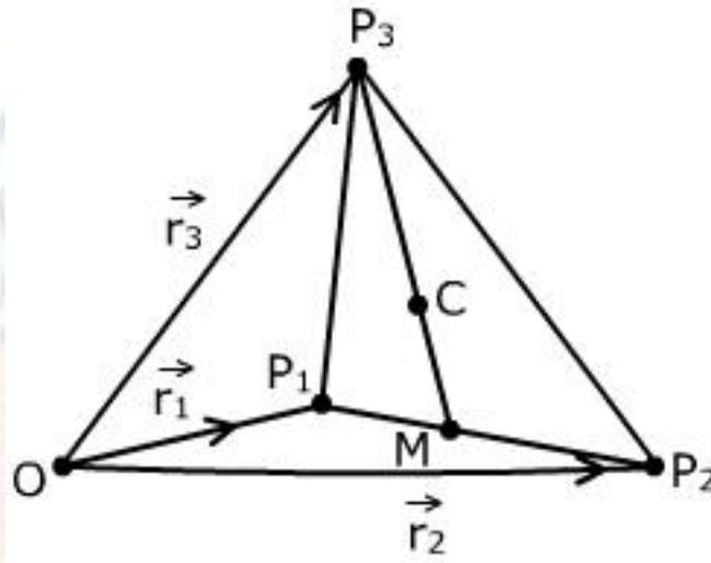
Fig. 2.4 Three equal masses placed at the vertices  $P_1, P_2, P_3$  of a triangle.
