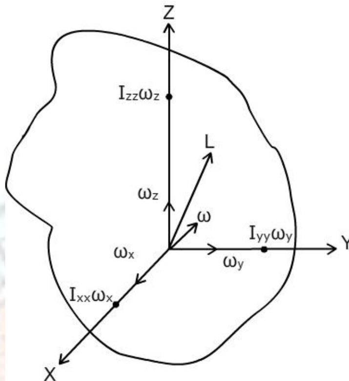
Fig. 5.3 An irregular body rotating about an axis where the angular velocity vector  $\omega$  is not along the angular momentum vector  $L$ .
