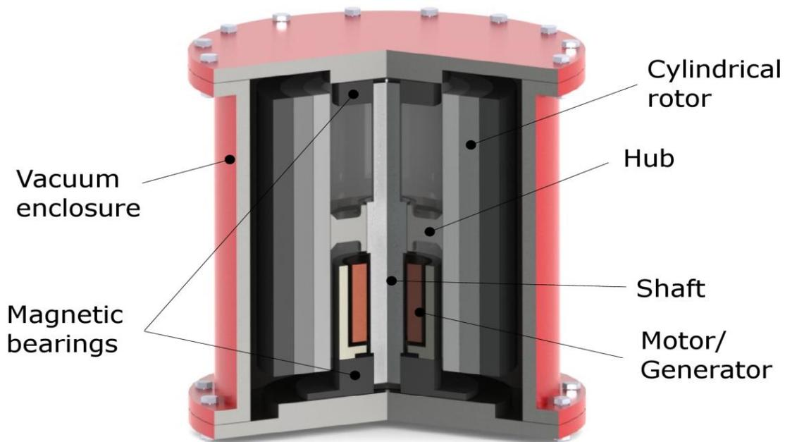
**Description English:** This image shows the main components of a typical cylindrical flywheel rotor assembly.
